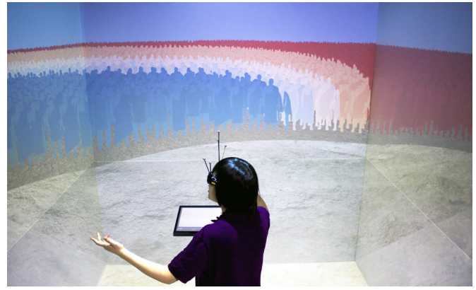
Figure 6: The first person real-time visualization of speech intelligibility shown within Pnyx III.
