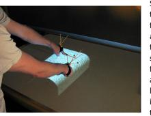
**Figure 4**. Using 6-DOF trackers attached to the hands, a surface fold is performed by defining a fold axis via 2D touch input.
