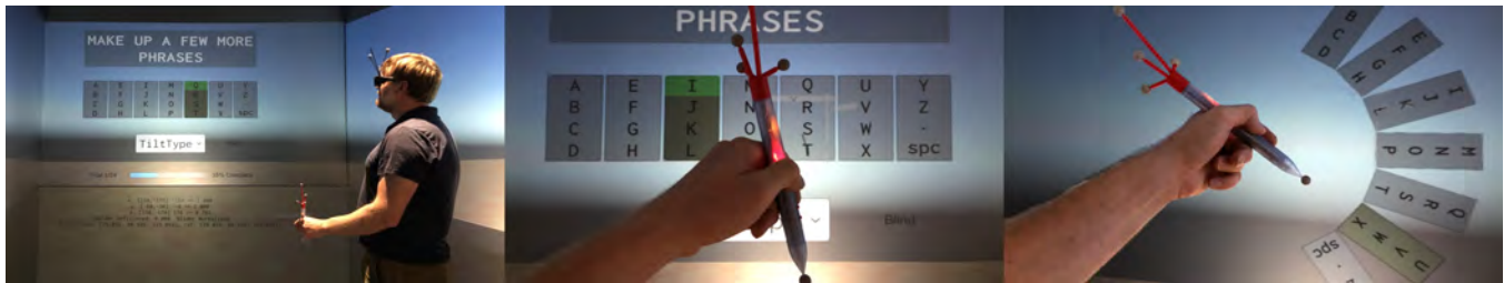
Figure 1: Left: A user manipulates a pen-shaped stylus to enter text in a virtual reality CAVE, where traditional keyboard interaction limits mobility. Center: The Tilt-Type interface uses small finger motions to tilt the stylus along two axes, changing the selected character in a binned layout. Right: The Arc-Type interface uses a rotational gesture and interactions with a touch slider to select characters from a radial layout.
